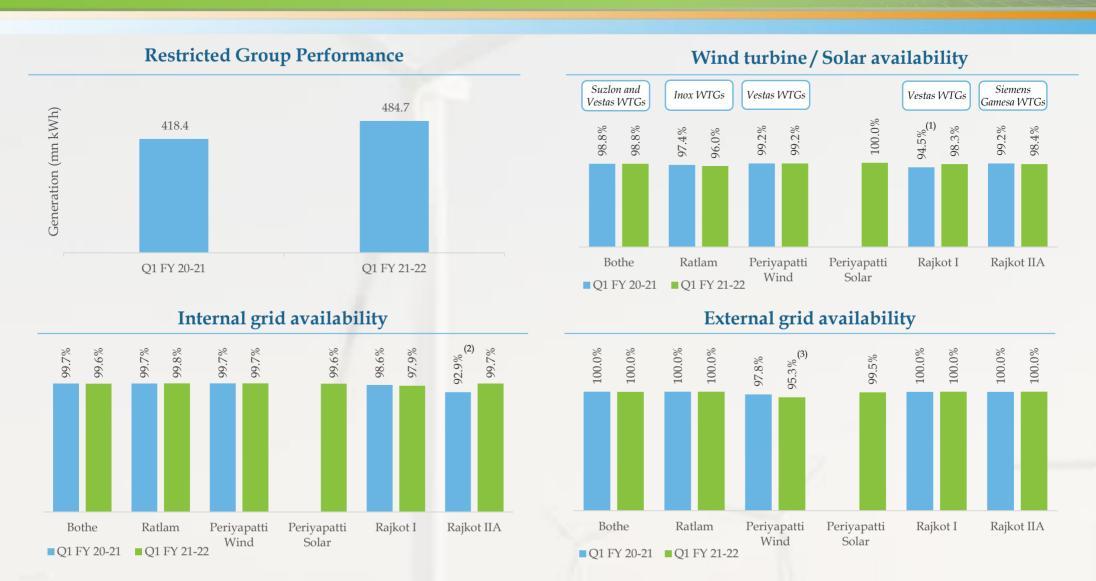
Periyapatti Solar started supply of power from 1st Mar-21. The Performance Ratio for the solar farm was 81.3% for Q1 FY 21-22
